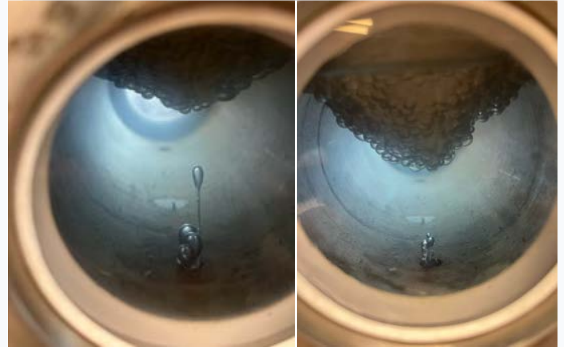
Figure 1: Visual confirmation of hydrate formation at 800 Psi and 1°C.
